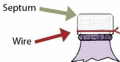
Fig. 4A Septa wired to vessel
