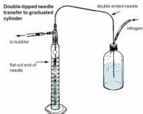
Fig. 3B Double-tipped needle transfer to graduated cylinder
