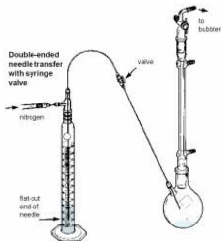
Fig. 3C Double-ended needle transfer with syringe valve
