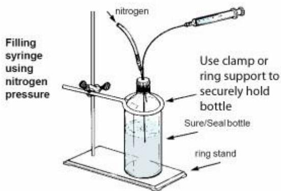
Fig.2A Filling syringe using nitrogen pressure
