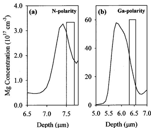
FIG. 2. Mg concentration profiles for (a) N polarity and (b) Ga polarity exhibiting evidence of surface accumulation layers. The Mg shutter opening and closing are shown schematically. Both layers were grown at a substrate temperature of 650 °C and a Mg source temperature of 300 °C.
