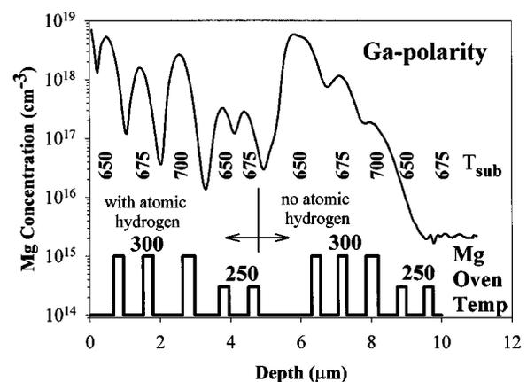
FIG. 1. Mg concentration in a Ga-polarity step-doped GaN layer. The Mg shutter opening and closing are shown schematically.
