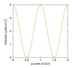
Scattering from 2 electrons separated by  $\vec{r}$  when  $\vec{q}$  is in the same direction as  $\vec{r}$ .
