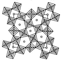
The structure can be constructed from the perovskite lattice through suitable crystallographic shear. Compare with the hexagonal tungsten bronze structure of the previous class.
