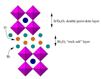
These are *intergrowth* phases comprising double "rock-salt" like  $Bi_2O_2$  layers intergrown with perovskite layers. The general formula of this family of phases is  $Bi_2A_{n-1}B_nO_{3n+3}$ ; n=1, 2, 3... The A site is like the A site in the perovskite structure, and the B site is like the B site in the perovskite structure. Typically, A = Pb, Bi, Na, K, Ca, Sr or the rare-earths, and B = Ti, Nb, Ta, Mo, W *etc.*
