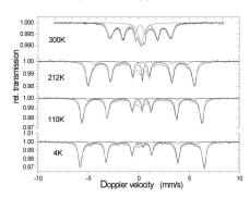
Note the changes in the nature of the Mößbauer spectrum at different temperatures, due to the changing internal fields in the magnetic system.
