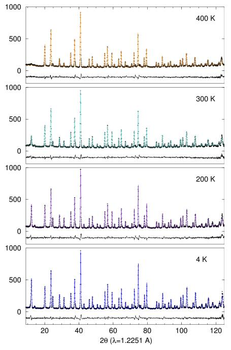
The neutron diffraction pattern also shows the emergence of a low angle line as the sample is cooled. This is due to the onset of collective magnetism. Analysis of the low-T patterns suggested that Cr and Fe spins are aligned in a ferrimagnetic manner (actually, the Fe spins are canted in addition).
