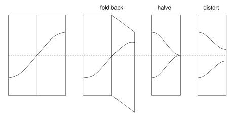
The dotted line is the Fermi energy. The Peierls distortion is an example of symmetry-breaking lifting a degeneracy. The Jahn-Teller distortion in d orbital solids is another such example.
