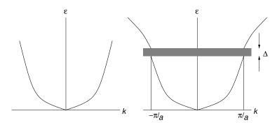
On the left is a sketch of the free electron wave function and on the right is a sketch of the effect of imposing a lattice on the free electron wave function with lattice parameter a.<sup>1</sup> At the k points  $k = \pm \pi/a$ , an energy gap  $\Delta$  opens up.
