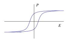
As is true for ferromagnets, the hysteretic behavior is a consequence of the presence of domains in the material.
