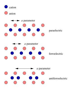
An example of an antiferroelectric is  $PbZrO_3$ , which is cubic  $(Pm\overline{3}m)$ , paraelectric above 503 K. Below this temperature, a combination of two effects, the tendency of the  $ZrO_6$  octahedra to tilt as a consequence of the tolerance factor being less than 1, and the tendency of the  $Pb^{2+}$  ions to go off-center, result in the antiferroelectric, orthorhombic crystal structure.
