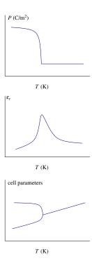
At the origins of such a phase transition are developments of a dipole within the unit cell, due to the centers of positive and negative charges not coinciding:
