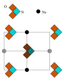
Room temperature ferroelectric structure of NaNO<sub>2</sub> projected on (001). The rigid NO<sub>2</sub> groups have been shown as little chevrons, and the Na<sup>+</sup> ions as circles. Hatching indicates that the atoms are at a height of -1/2.
