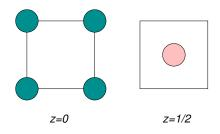
**ZnS** (zinc blende): ZnS is also found in the wurtzite structure. In cubic (blende) ZnS, the cell parameter is 6.23 Å. Note the 4-4 coordination, and the relation to the diamond crystal structure. Other examples are AgI, AlAs, AlP, AlSb, BAs, BN, BP, BeS, BeSe, BeTe, CdS, CuBr, CuCl, CuF, CuI, GaAs, GaP, GaSb, HgS, HgSe, HgTe, INAs, InP, MnS, MnSe, SiC, ZnSe, ZnTe.
