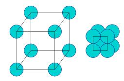
Two views of the simple cubic structure. In the second view, on the right, the atomic spheres are shown touching each other. Verify that there is only one atom per unit cell by noting that the 8 atoms at corners are all only 1/8th within the cell. In other words, the 8 atoms are each shared between 8 cells.
