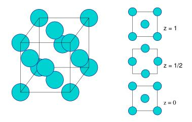
The structure is a bit crowded so we also draw it as sections along the z axis. Note that the cell parameter a is given by  $\sqrt{2}a = 4r$ , and that there are four atoms per unit cell. The packing efficiency
