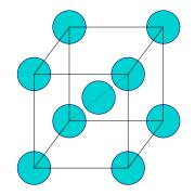
There are now two atoms in the unit cell. The one in the center is not shared with other cells, while the 8 in the corner are each shared with 8 other cells; the total is 1 (center) +  $8 \times \frac{1}{8}$  (corners) = 2. If the atomic spheres touch each other, we observe that the
