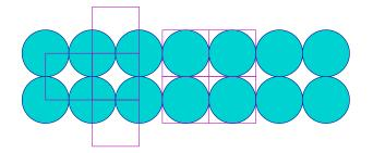
Note that there is again one disk per unit cell. The packing efficiency is now:
