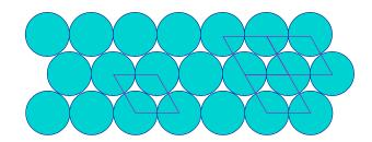
Note that there is one disk per unit cell. Calculate the packing efficiency (the ratio of area taken up by the disks to the area of the unit cell) of this structure, and verify that it is:
