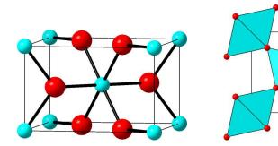
Left: The rutile structure showing the TiO<sub>6</sub> octahedron within a single unit cell.
