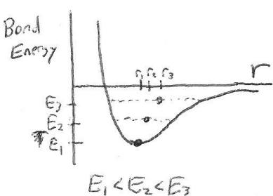
As a crystal is heated, the energy in the crystal increases. This energy causes the atoms to vibrate. The distance it can vibrate is shown by the walls of the well in the Potential Energy curve. The material expands because the walls of the well are assymetric so the mean distance  $r$ , is larger for increasing T's.
