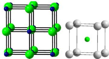
Under pressure, NaCl in the NaCl structure transforms to the CsCl structure, going from CN = 6 to CN = 8: Non-directional solids are not terribly particular about CN.
