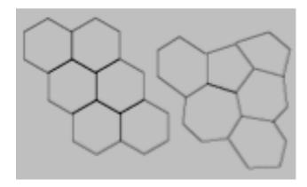
Schematic arrangements of atoms in a planar crystal (left) and glass (right). Note that the coordination numbers of the atoms (CN = 3) remains the same.
