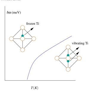
The frequency (energy) of the soft mode goes to zero as the phase transition is approached.
