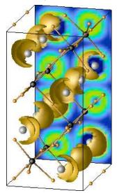
In this depiction of the crystal structure of PbZrO<sub>3</sub>, the "lone pairs" on the Pb atoms are visualized using DFT calculations of the electronic structure. Note that the "lone pairs" creates a structural distortion that cancels itself.
