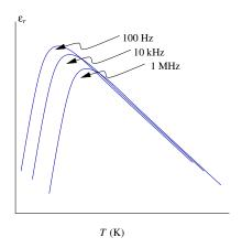
• Relaxors are useful since they have a high dielectric constance even at radio frequencies and they saturate at low voltages. Because of the broad phase transition, the T dependence of  $\epsilon_r$  does not create problems in devices. In addition, the hysteresis is small, the energy densities are high and the materials are field-tunable.
