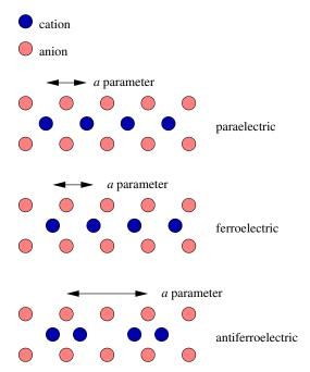
• An example of an antiferroelectric is PbZrO<sub>3</sub>, which is cubic  $(Pm\overline{3}m)$ , paraelectric above 503 K. Below this temperature, a combination of two effects, the tendency of the ZrO<sub>6</sub> octahedra to tilt as a consequence of the tolerance factor being less than 1, and the tendency of the Pb<sup>2+</sup> ions to go off-center, result in the antiferroelectric, orthorhombic crystal structure.
