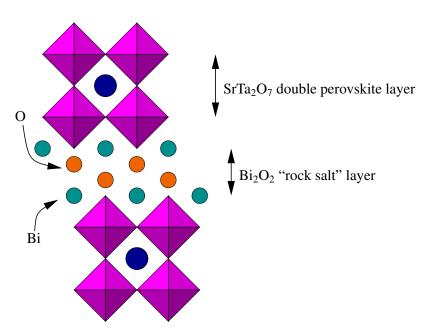
These are *intergrowth* phases comprising double "rock-salt" like  $Bi_2O_2$  layers intergrown with perovskite layers. The general formula of this family of phases is  $Bi_2A_{n-1}B_nO_{3n+3}$ ;  $n=1, 2, 3 \dots$  The A site is like the A site in the perovskite structure, and the B site is like the B site in the perovskite structure. Typically, A = Pb, Bi, Na, K, Ca, Sr or the rare-earths, and B = Ti, Nb, Ta, Mo, W *etc*.
