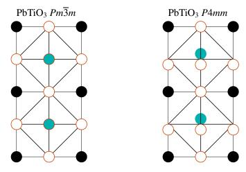
• In the particular case of PbTiO<sub>3</sub>, the phase transition from the cubic, paraelectric phase to the tetragonal ferroelectric phase (a displacive phase transition) is associated with the freezing of a phonon mode that is referred to as the "soft mode". Phonon modes are specific vibrational modes of the crystal lattice. In the case of PbTiO<sub>3</sub>, this phonon mode is associated with the Ti atom in the center of the octahedron:
