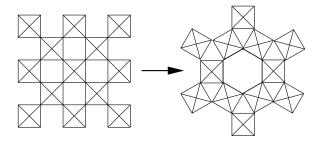
An example is the phase transition from the perovskite lattice (left above) to the hexagonal tungsten bronze structure (right above). The A atoms in the structure are not shown.
