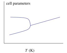
• At the origins of such a phase transition are developments of a dipole within the unit cell, due to the centers of positive and negative charges not coinciding:
