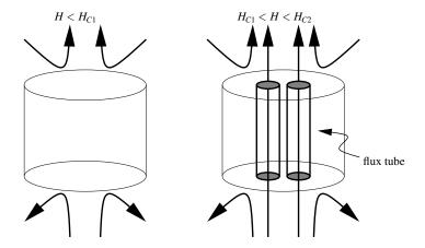
Examples of type II superconductor are most superconducting alloys and intermetallics (such as the so-called A15 compounds) and the high  $T_C$  copper oxide superconductors. The record for the second highest critical field  $H_{C2}$  is held by the Chevrel phase PbMo<sub>6</sub>S<sub>8</sub> of 54 T at 4 K. Such materials are good candidates for forming superconducting solenoids.
