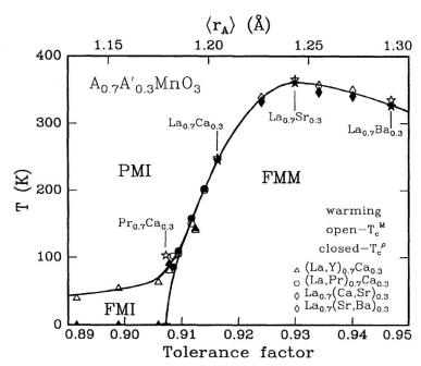
From H. Y. Huang *et al. Phys. Rev. Lett* **75** (1995) 914. This plot shows the temperature at which the different compounds become ferromagnetic as a function of the average size of the A cation. The tolerance factor t, and the average 9-coordinate Shannon-Prewitt radii form the different ordinate (x) axes. Note how the highest transition temperature is found for a specific tolerance factor. PMI = paramagnetic insulator, FMM = ferromagnetic metal, FMI = ferromagnetic insulator.
