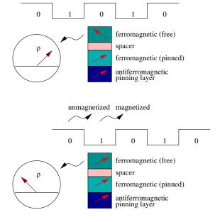
When the head (the free ferromagnetic layer) runs over a magnetized region on the hard disk, the magnetization of the magnetic layer is aligned with the magnetization of the pinned magnetic layer. This reduces the electrical resistivity of the assembly.
