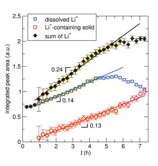
Integrated area of solid increases linearly with discharge
