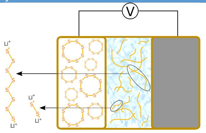
S<sub>2</sub><sup>2-</sup> near the cathode can further reduce to create Li<sub>2</sub>S, adding to the capacity
