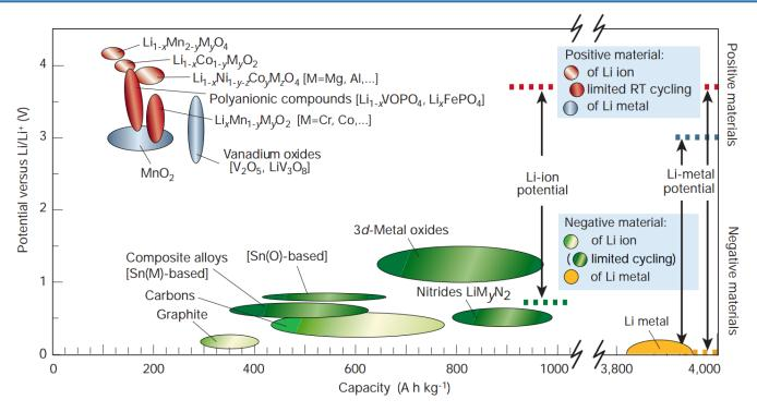
Graphite (typically used in Li–ion batteries) has a theoretical specific capacity of 372 mAhg<sup>-1</sup> (operating capacity of ~350 mAhg<sup>-1</sup>) which is incompatible with a sulfur cathode
