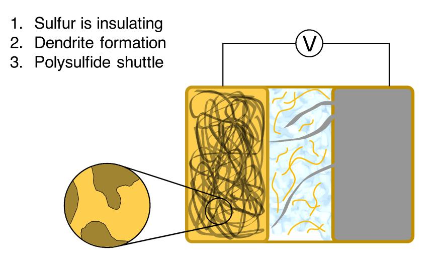
Chains of diradical sulfur and their counter lithium cations solubilize in the liquid electrolyte during discharge, causing capacity fade
