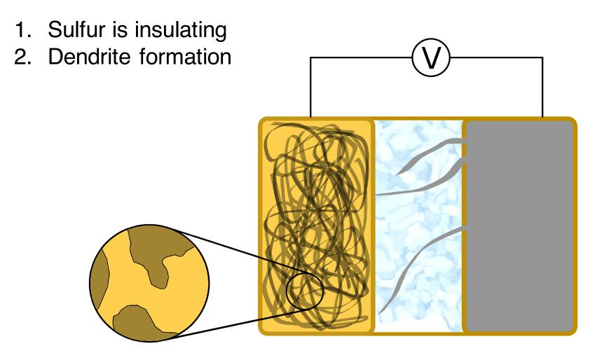
Dendrites can be atomically thin fibers of Li that extend from the anode to the cathode over many cycles and cause short-circuiting + safety concerns
