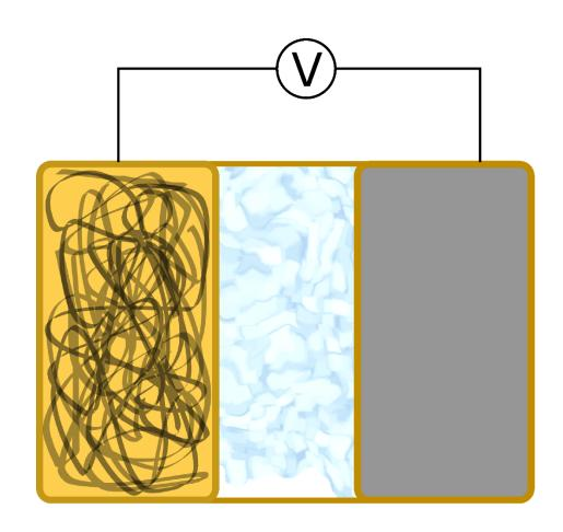
The cathode must include a mixture of conducting carbon and sulfur to get sufficient charge and ion mobility needed for battery cycling
