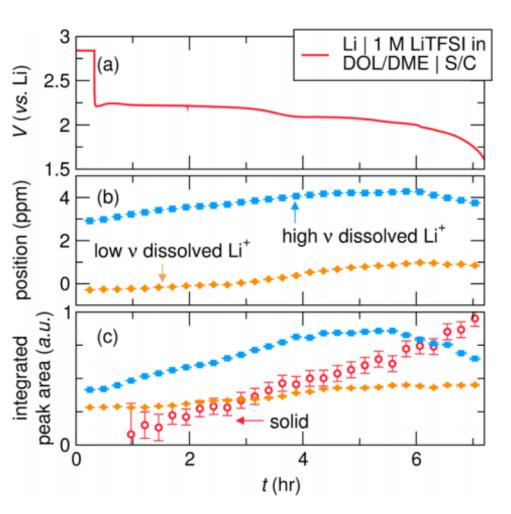
High frequency Li<sup>+</sup> = closer to cathode High concentrations of Li<sup>+</sup> cause a positive shift in resonance
