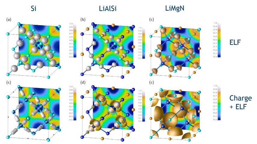
Electron localization functions of the 8e compounds show strongly localized bonding.
