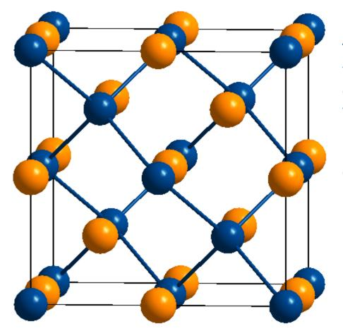
The Zintl-Klemm concept and valence compounds: The example of LiAl (Li<sup>+</sup>Al<sup>-</sup>). Al<sup>-</sup> is isoelectronic with C and forms a diamond lattice. The Li<sup>+</sup> ions stuff the Al<sup>-</sup> lattice. Note the 8 electron rule operates.
