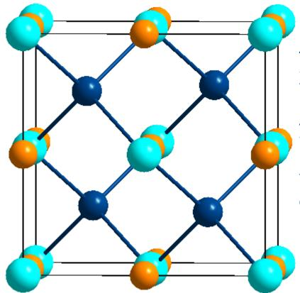
The half-Heusler crystal structure: XYZ. 3 interpenetrating fcc lattices.
