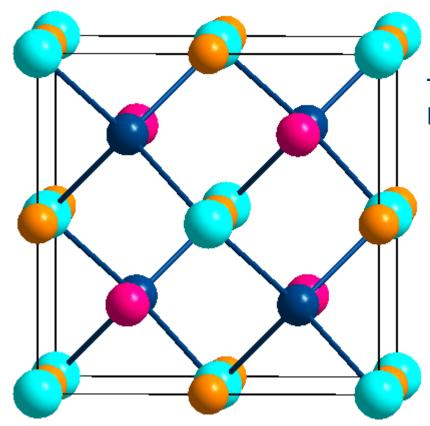
The Heusler crystal structure: XY<sub>2</sub>Z F. Heusler (1903) 4 interpenetrating fcc lattices.
