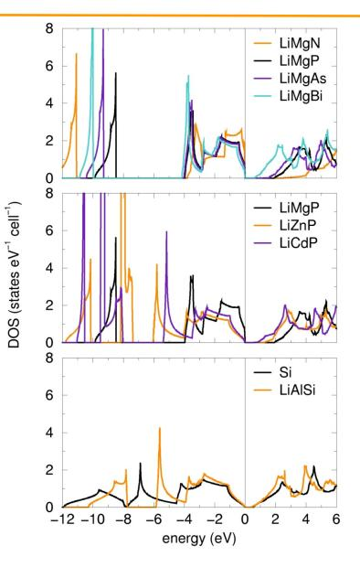
LMTO DOS of 8e half-Heulsers indicates a strong dependence of the band gap on composition of the zinc-blende lattice.
