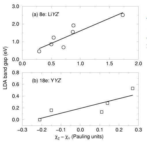
The band gaps of some 8e and 18e half-Heuslers depend on the electronegativity of the ions in the zinc-blende framework.
