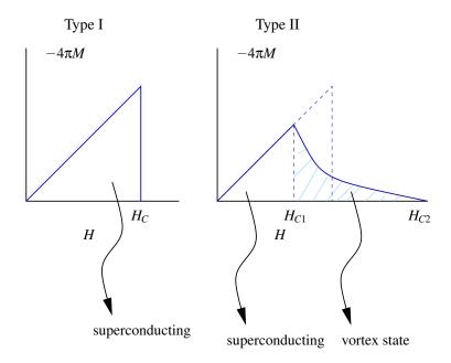
In type I superconductors (pure metals), the superconductivity is destroyed by small magnetic fields; above some critical magnetic field  $H_C$ , the material is no longer superconducting. Typical critical fields are of a 1000 Oe.
