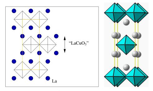
The large spheres are the  $La^{3+}$  ions. The formula suggests that in  $La_2CuO_4$ , Cu is in the +2 oxidation state.  $Cu^{2+}$  has 9 d electrons. Since it is octahedral, we would expect the crystal field diagram and the DOS to look as follows:
