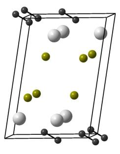
Projection of the monoclinic  $Y_2C_2Br_2$  structure almost down the b axis, showing carbon atoms (black) occurring as covalently bonded pairs, metallic Y (gray) and ionic Br (olive). Simon *et al.*, *Z. Anorg. Allg. Chem.* **622** (1996) 123.
