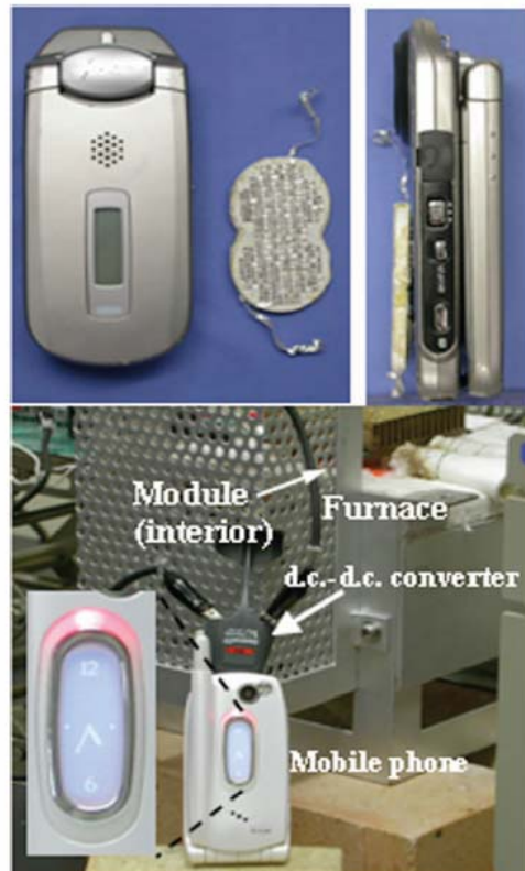
FIG. 4. (Color) Comparative photographs of the oxide module and a mobile phone, and a demonstration of charging a lithium-ion battery in the mobile phone. Red LED on the mobile phone indicates charging of the lithium-ion battery is in progress.
