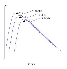
• Relaxors are useful since they have a high dielectric constance even at radio frequencies and they saturate at low voltages. Because of the broad phase transition, the T dependence of  $\epsilon_r$  does not create problems in devices. In addition, the hysteresis is small, the energy densities are high and the materials are field-tunable.
