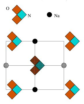
Room temperature ferroelectric structure of NaNO<sub>2</sub> projected on (001). The rigid NO<sub>2</sub> groups have been shown as little chevrons, and the Na<sup>+</sup> ions as circles. Hatching indicates that the atoms are at a height of -1/2.
