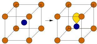
Sketch displaying the tendency of a lone pair ion (blue) such as  $Pb^{2+}$  to go off-center in its coordination polyhedron, leaving in the center of the polyhedron, the  $s^2$  lone pair. Such a sketch is quite accurate for describing the crystal structure of PbO in the litharge modification.
