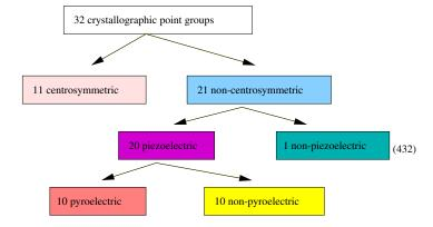
$\bullet$  The ferroelectric phase transition (for example, in PbTiO<sub>3</sub>) is characterized by the development of a spontaneous (zero field) polarization, changes in the dielectric constant, and crystal structural changes.:
