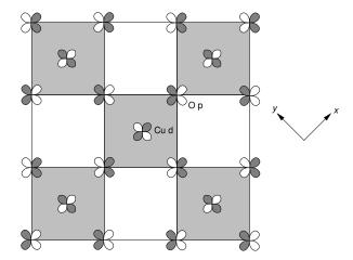
Sketch out the band structure of such a 2D lattice, concentrating on the band formed through the metal-oxygenmetal network (nearest neighbors). Suggest why similar compounds formed from *early* transition metals such as Ti or V would not have bands that are as disperse.<sup>1</sup>.
