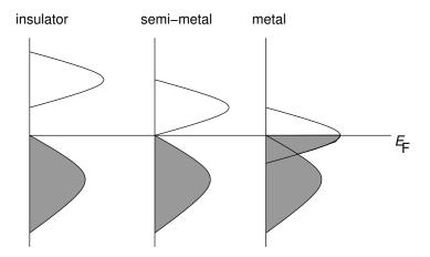
Electrons in filled bands do not carry a current because they cannot move without violating Pauli's exclusion principle. If they do move, their motion must be compensated by the motion of a hole in the same direction, or of an electron in the opposite direction.
