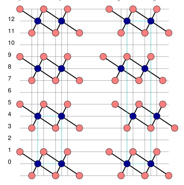
On the left is the structure of  $CdI_2$  projected down the b axis and on the right is the structure of  $CdCl_2$ . The cyan-colored box marks the unit cell.
