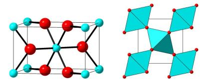
Left: The rutile structure showing the TiO<sub>6</sub> octahedron within a single unit cell.
