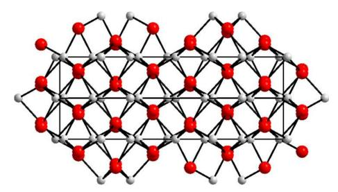
The corundum structure with the c axis going from left to right. Red spheres are O and grey are Al.
