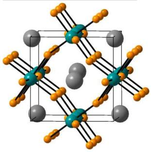
Here is the structure looking down the long c axis. The connectivity of the perovskite structure, namely the corner-shared octahedra are clearly seen. The large grey atoms are Ca.
