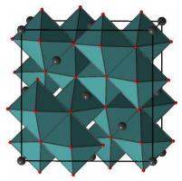
The structure can also be regarded as being formed by strips of edge-sharing octahedra that are laid down forming a trellis. Tetrahedral voinds in formed by these strips of octahedra are where the Mg sit.
