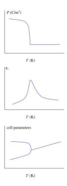
At the origins of such a phase transition are developments of a dipole within the unit cell, due to the centers of positive and negative charges not coinciding:
