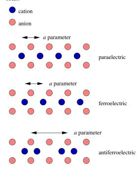
An example of an antiferroelectric is  $PbZrO_3$ , which is cubic paraelectric above 503 K. Below this temperature, it is orthorhombic and antiferroelectric. orthorhombic
