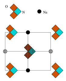
Room temperature ferroelectric structure of  $NaNO_2$  projected on (001). The rigid  $NO_2^-$  groups have been shown as little chevrons, and the  $Na^+$  ions as circles. Hatching indicates that the atoms are at a height of -1/2.
