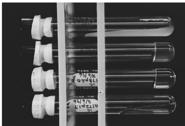
FIG. 3. Series of test tubes filled with 1b based mixtures of different compositions. From bottom to top increasing \Phi_w . c_{\text{PEG}} = [\text{mole PEG-surfactant}/(\text{mole PEG-surfactant} + \text{mole DMPC})] \times 100 . Bottom sample: \Phi_w = 0.72 and c_{\text{PEG}} = 1.9 in the fluid L_\alpha -phase; second sample: \Phi_w = 0.78 and c_{\text{PEG}} = 2.0 in the L_{\alpha,g} gel phase; third sample: \Phi_w = 0.85 and c_{\text{PEG}} = 2.1 in the L_{\alpha,g} gel phase; top sample: \Phi_w = 0.92 and c_{\text{PEG}} = 2.0 in the two phase region.
