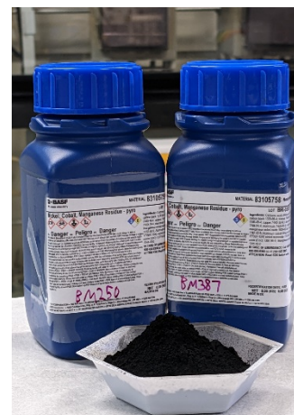
'Black Mass' is the complex mix of compounds resulting from carbothermal reduction of LIBs
