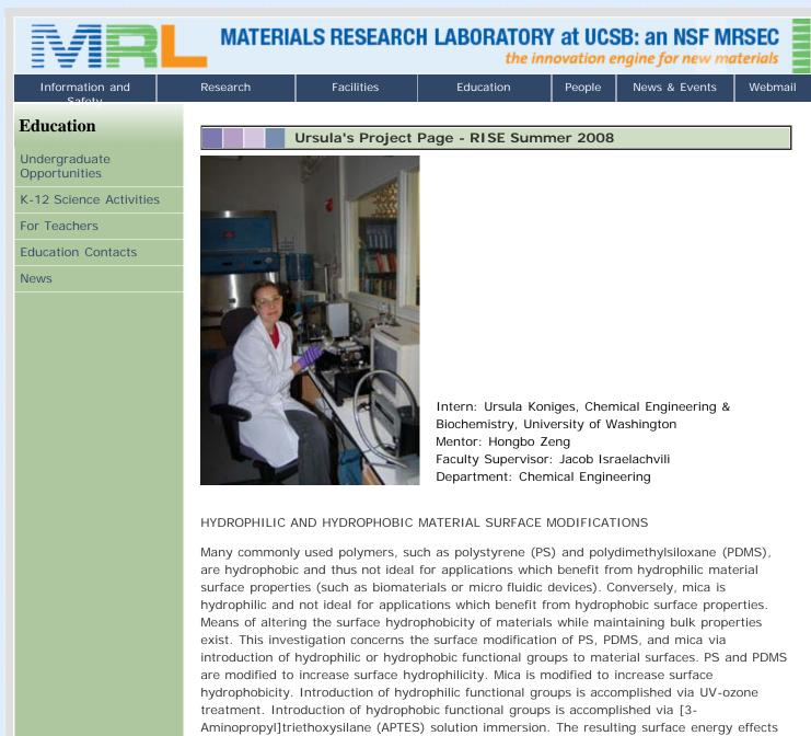
Aminopropyl]triethoxysilane (APTES) solution immersion. The resulting surface energy effects are examined using sessile drop contact angle analysis. Surface forces apparatus (SFA) is used to measure deposited APTES monolayer thickness. Results indicate successful achievement of desired surface modifications.
