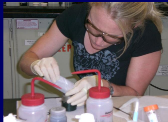
Poured powder into 13 mm die for pressing 1.0 g pellets
