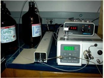
2. Large molecules move faster than smaller ones on the columns.
