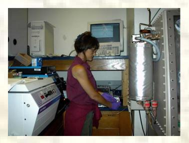
1. Polypeptide is dissolved in DMF, filtered, and injected onto the columns.
