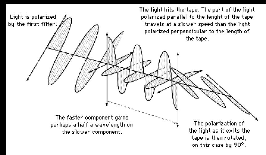
A wave diagram of polarized light passing through a birefringent tape.
