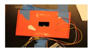
6. NOTE: This depends on color of alligator clips. Y= yellow, R= red, and W= white. Pre-connect your 1st shade by clamping alligator clips (ex: Y=ground, R=5V, W=sensor) such that Y and R are opposite each other, and W is attached in the center.
