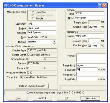
and reference crucibles. Users may then run their sample, using the same crucibles, as the "Sample+Correction" option and the correction (baseline) will be automatically removed from the data. The correction measurement data is retained and may be viewed in the analysis program Proteus. Without a recent correction file the Sample+Correction option will be grayed out and not selectable.
