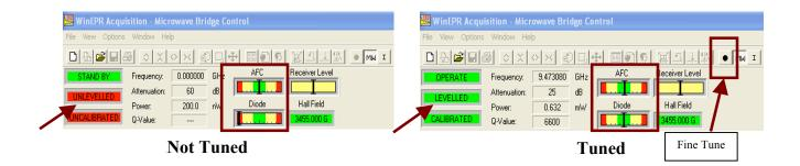
If the AFC and Diode are not exactly in the center, then you can hit the **Fine Tune** button.
