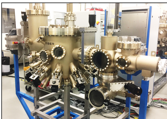
Fig. 17. The molecular beam epitaxy chamber for topological crystalline insulator growth awaiting installation in the PI's lab.
